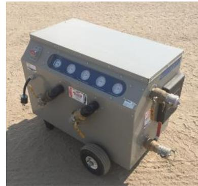
Figure 10 - Plate Heat Exchanger Unit
