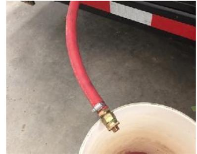
Figure 32 - Fill/Drain Hose
